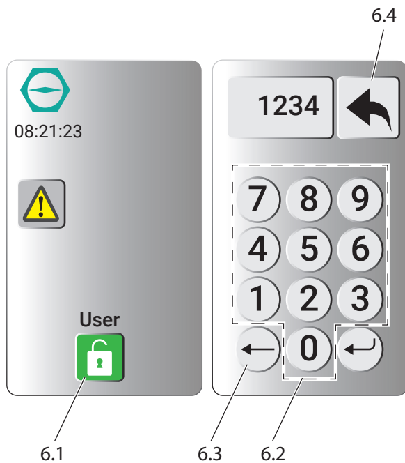
Figure 2. Memory system display – logging in and save working position (actual product may vary from figure)
